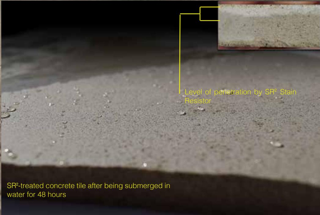
Level of penetration by SR<sup>2</sup> Stain Resistor
